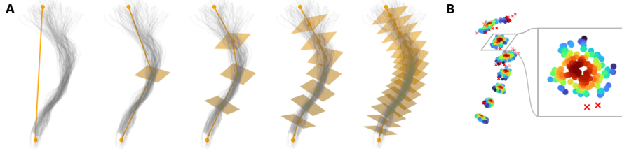
Figure 2.4: Visualization of the filtering process for pathway deviations. A An average bundle trajectory is iteratively computed. B At each step, outlier streamlines (red crosses) are identified based on their position density on the plane perpendicular to the trajectory.
